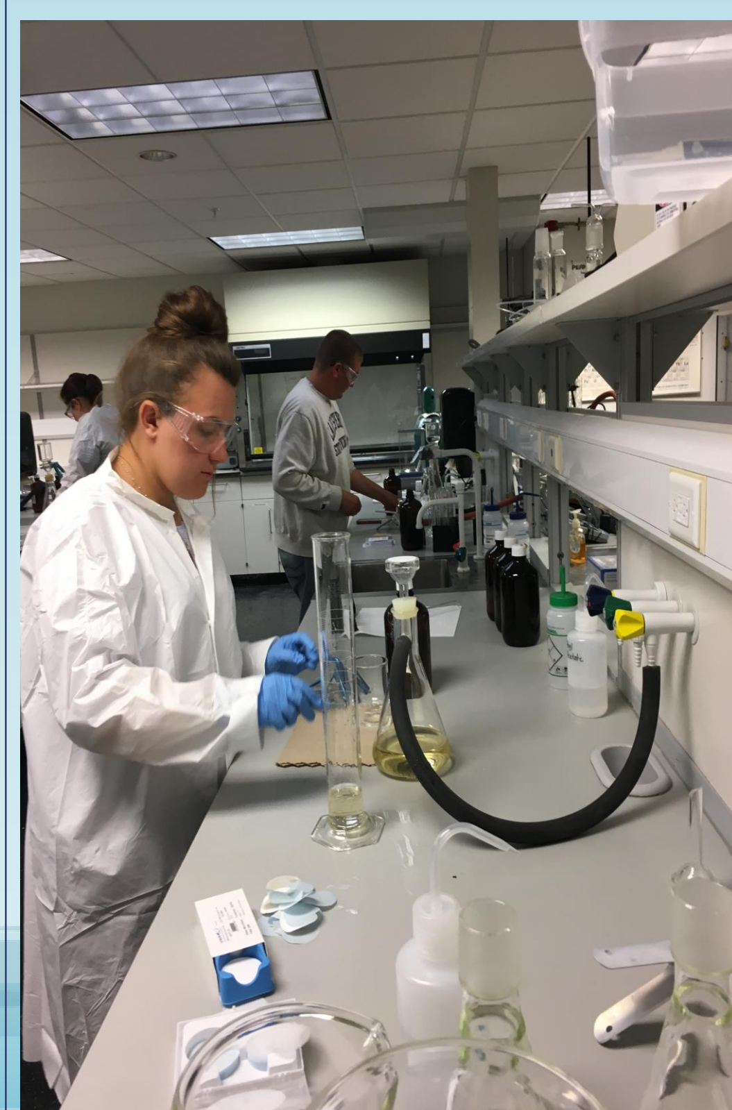
Figure 2. Student researcher, Claryn Sangster, processes water samples through Sigma Millipore filters at Lake Superior State University Environmental Analysis Lab.
